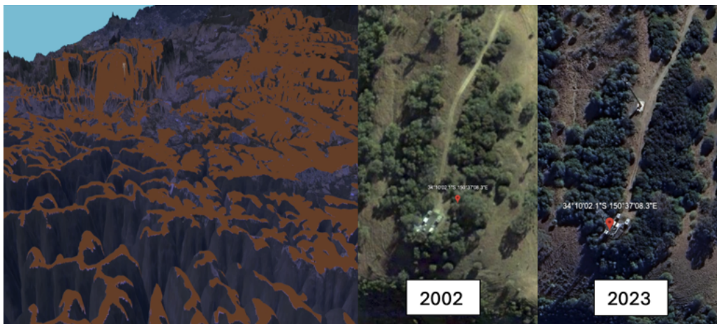
Figure 6.6.0.1: (left) Line of Sight (LOS) RF analysis for Picton Base Station in 2001 in 3D looking north and down at a height; (right) Satellite imagery comparisons between 2002 and 2023 of the same Picton base station site
