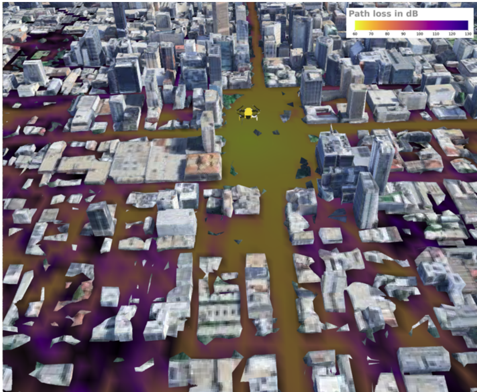
Figure 6.4.7.1: RF coverage for one drone in the Adelaide CBD above Victoria Square with an omnidirectional antenna
