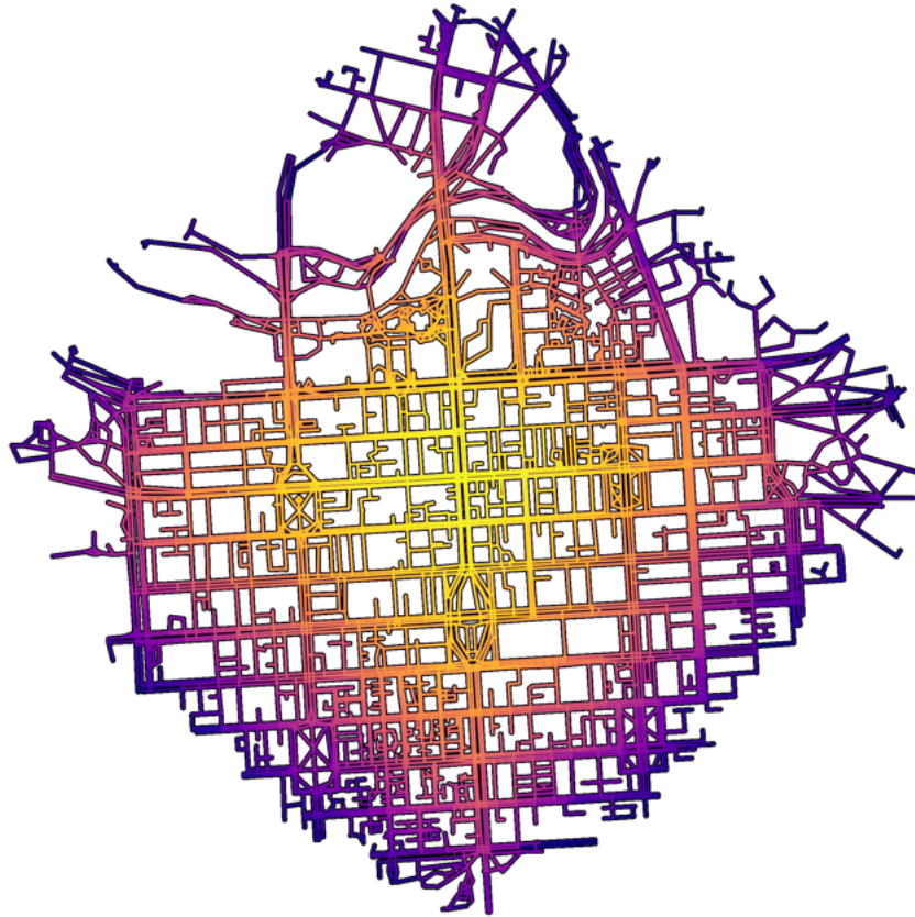
Figure 4.3.2.1: Shortest path tree (SPT) example for a pedestrian in Adelaide CBD
