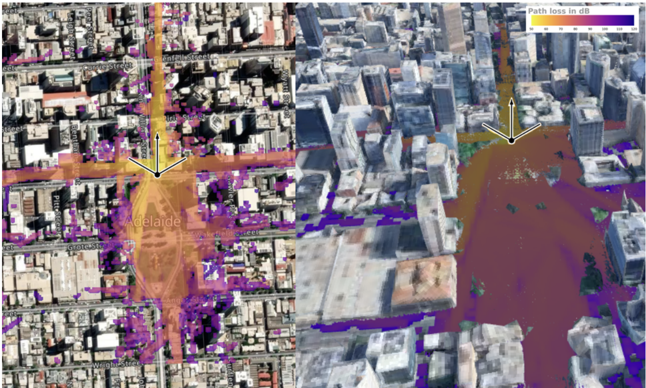
Figure 5.5.7.1: (left) 2D bird's-eye view of RF ray traced map of Google 3D tiles data using Sionna RT for a north-facing transmitter located at Victoria Square; (right) Same heatmap overlaid onto the Google 3D tiles data
